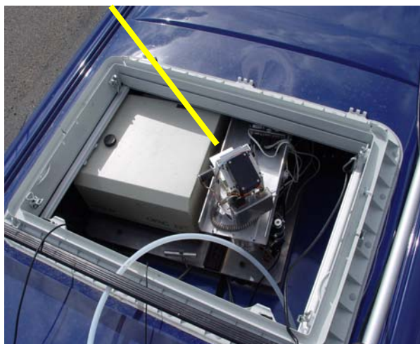
Fig. 1. The SOF instrument positioned in a VW transporter. The device in the lower figure tracks the sun.
